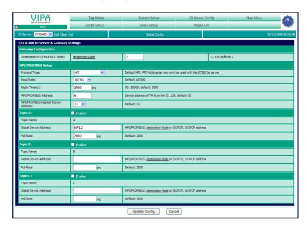
At "Gateway Configuration" and "MPI/Profibus Setup" the values are preset, which are to be used per default.
