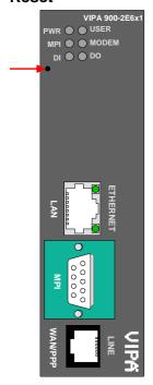
A reset at the Teleservice module may be initiated by the Reset button. The Reset button is allocated below the LEDs behind an opening. Please use for operation a pointed object.
